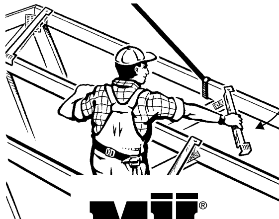
For trusses 12000 mm to 16000 mm 1 TrussSpacer at apex and at each top chord panel point - 3 per bottom chord
