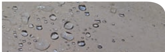
CCS penetrating sealers repel water while allowing the surface to breathe.
