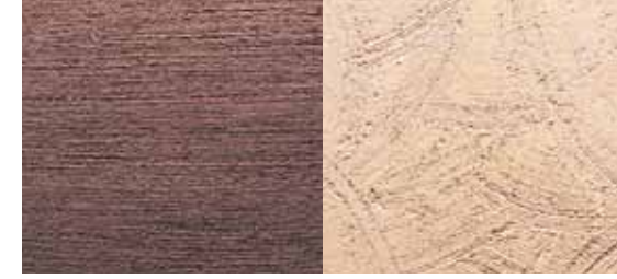
Broom Finish Trowel Finish
